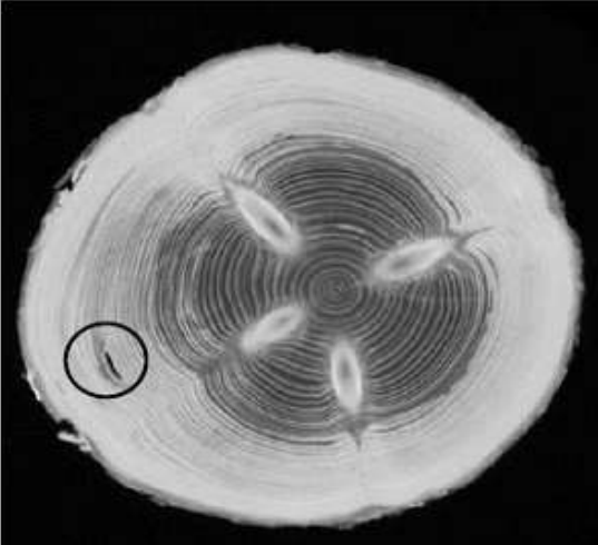
Resin pocket in sapwood
