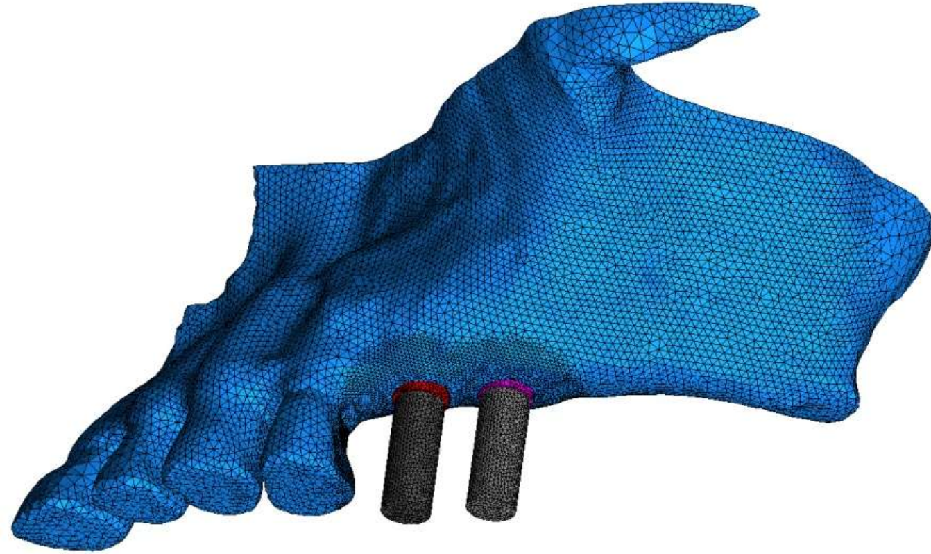
Fig. 14: Nodes in common at material transitions (maxilla/implant/abutment)
